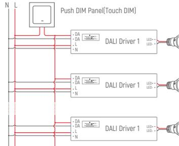
Remark: Only use open push button without indicator light. Maximum cable length between each Unit: 20 meters.
