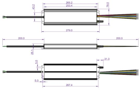
\*\*Input Rubber cable 3\*1.0mm² (VDE approval), the Y/G cable connect with (FG), Brown with AC (L), Blue with AC(N) (EU) Input SJOW Rubber cable 3\*18AWG (UL approval), the green cable connect with (FG), Black with AC (L), White with AC(N) (US)
